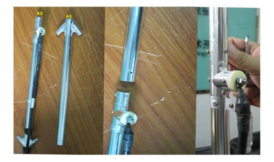
III. Connect and tighten elements B1 and B2 on the main elements(A &A2) through the following steps:
