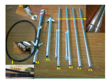
II. Install the main element of antenna, connect A1 on top of A2.
